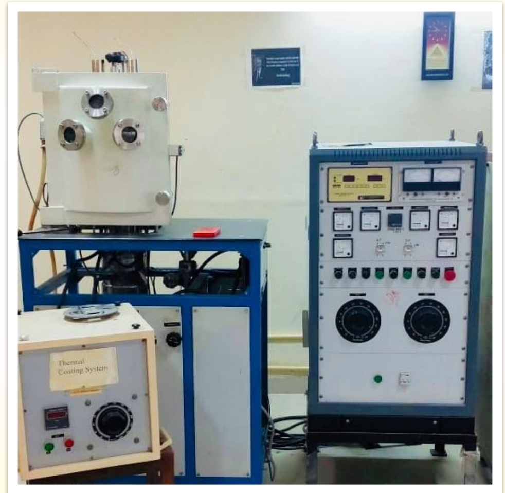
THERMAL VACUUM COATING UNIT
